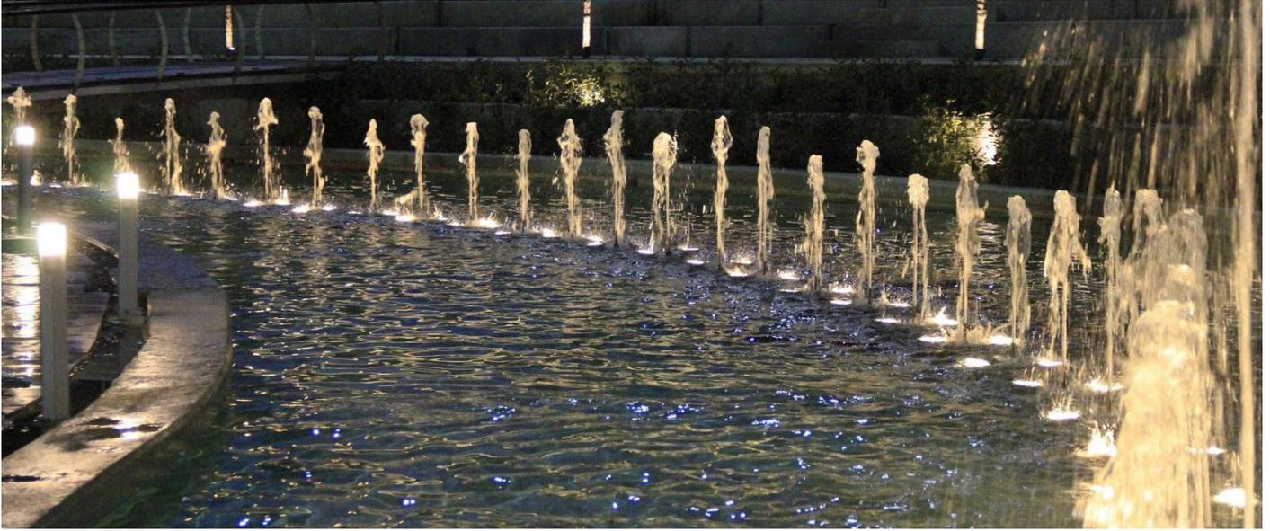
AquaSTAR is a mounted unit connected to a collector, designed to create captivating water displays. It offers lighting options such as 1 X AquaLIGHT C for added visual appeal. A single pump supplies water to the collector, while a solenoid valve under each nozzle controls the flow. By aligning nozzles in a line, you can achieve beautiful sequential running effects.
