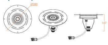
Top Plate thickness is 5mm. Top Plate Round Ø 280 with Top Plate Holder.
